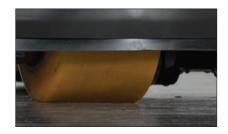
RUBBER BUMPER SKIRT Rubber skirting directs light debris away from the drive tire.
