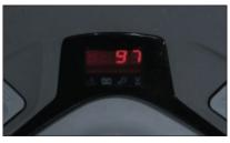
BATTERY DISCHARGE INDICATOR (BDI) WITH LIFT INTERRUPT
