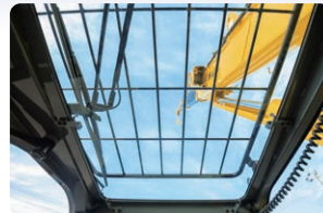
Wide View Roof Window
